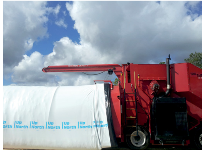
Figure 4. Bag silo filling.
